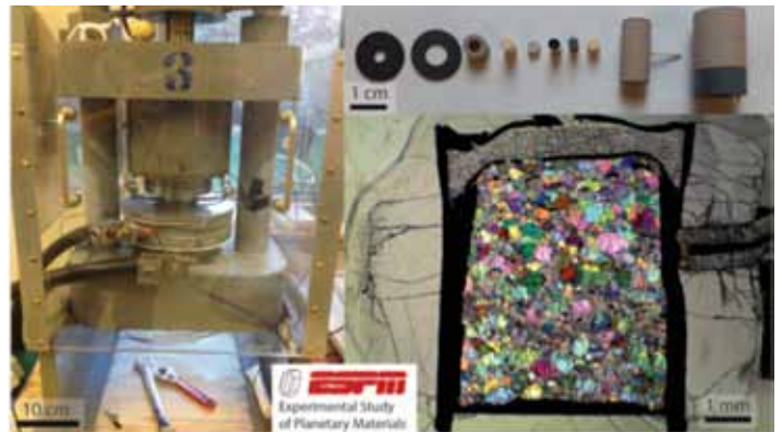
Fig. 2 – Griggs apparatus (left), assembly parts (upper right), and a thin section of a deformed sample (right).
