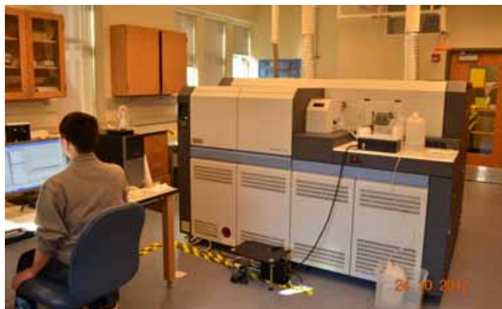
Figure 1: Graduate student Cheng Heng sitting at two-year old multi-collection inductively-coupled-plasma mass-spectrometer.
