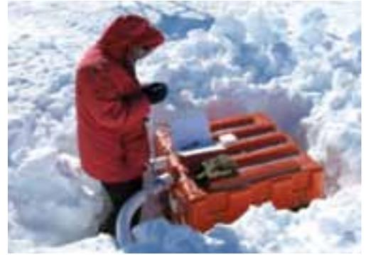
Figure 3: Turning the station on. All of the electronics were stored in insulated boxes to conserve heat.
